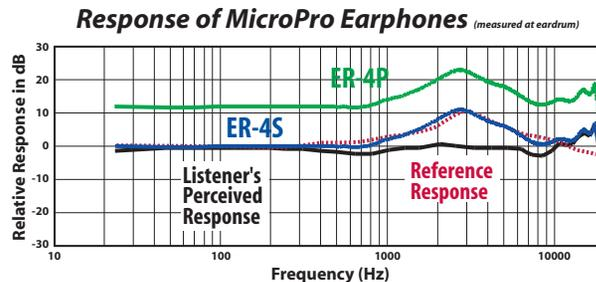
The above graph indicates that 4P earphones have 12 dB higher sound output and increased bass compared to the original ER-4S earphones. The dotted red line is the reference response of the open ear to live performances (CD equalization). The black line represents how a listener perceives the sound.
