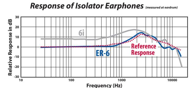
The above graph indicates that 6i earphones have 8 dB higher sound output and increased bass compared to the original ER-6 earphones. The dotted red line is the reference response of the open ear to live performances (CD equalization).
