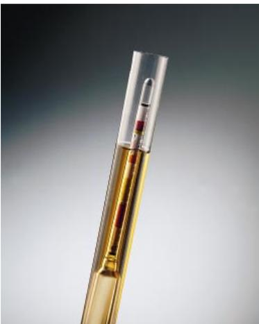
To check if your beer is ready to bottle, use your hydrometer to measure the specific gravity of the beer by half filling the tube with beer and checking the scale on the hydrometer. When ready, the final reading should be between 1.008-1.010 when using the Coopers/CSR brewing sugar provided in this kit.
